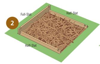
Finally, put the two remaining half-slats into position
